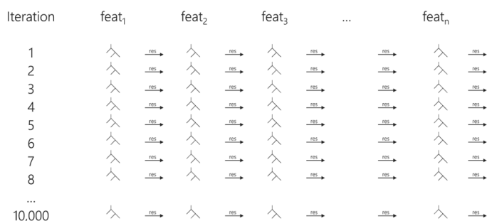
Figure 2. Explainable Boosting Machine Tree-Based Training Procedure
